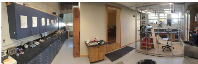
The New Mexico Highlands University Paleomagnetic-Rock Magnetic Laboratory equipped with a static 56 m 3 (front) and dynamic 15.6 m 3 (right) magnetically shielded rooms.
