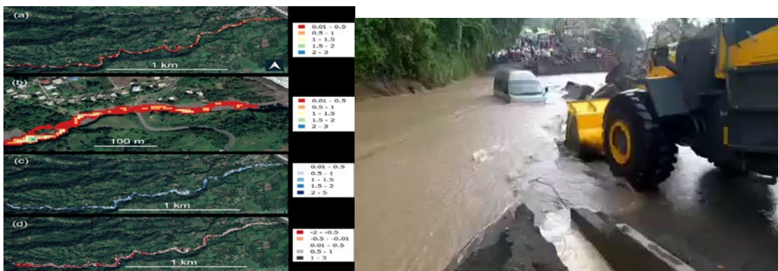
Left - A lahar at the Overland river crossing, October 2022 (shared on the Changing Landscapes WhatsApp group); Right - LaharFlow model simulations of lahars at the Overland crossing: (b) flow depth (m), (c) flow speed (m/s)
